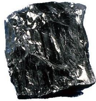
Fig. 1.4.b. Anthracite with a calorific value of 29 MJ/kg (source: Wikipedia)
