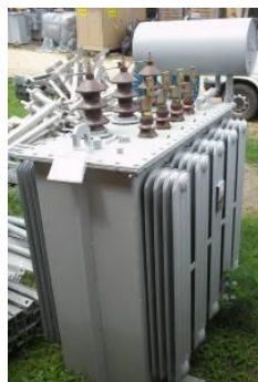
Fig. 3.4. Medium/low voltage transformer - 1
