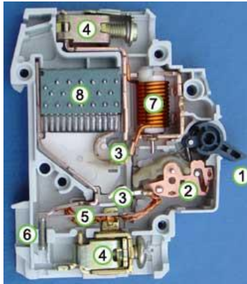
Fig. 6.8. Construction of an automatic fuse
